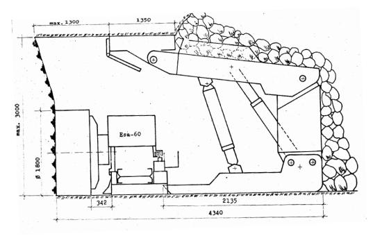
**Fig. 3.** Cross section of a longwall equipped with sublevel caving shields type VHP742/1 and ESA-60L shearer loader
