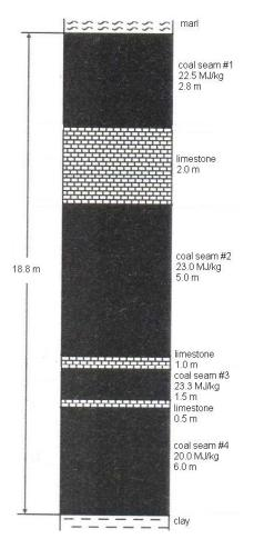
Fig. 4. Vertical section of the coal seams. Document prepared by the coal mine
