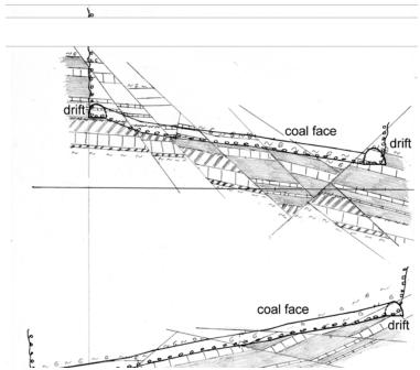
Fig. 1. Longitudinal sections of two longwalls, cutting mostly country rocks due to their momentary unfortunate position. Document prepared by the coal mine
