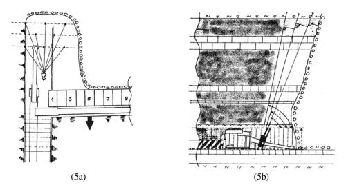
**Fig. 5.** Crossing of the longwall and the transportation drift (5a) and the vertical section of coal seams and the blastholes along the drift (5b)
